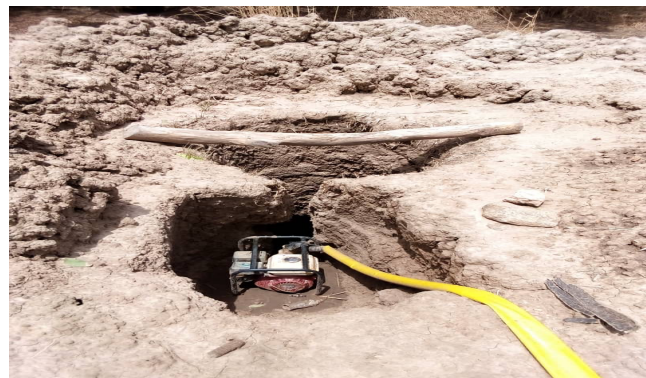
Figure 5. Shallow well in riverbank for motorized pump irrigation
