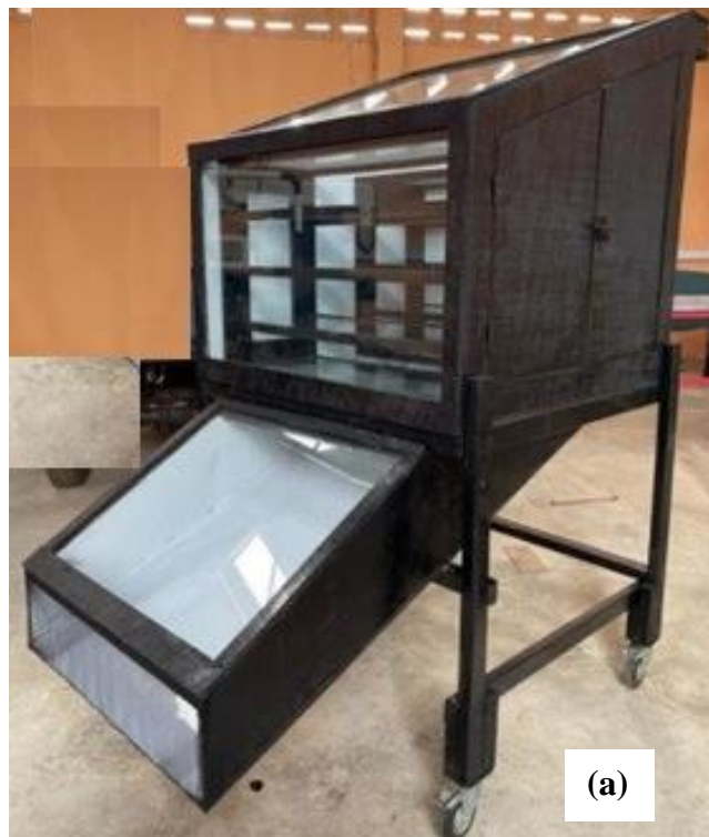
Figure 7. Pictures of the constructed MMNC Solar Dryer (a) Doors closed (b) Doors closed
